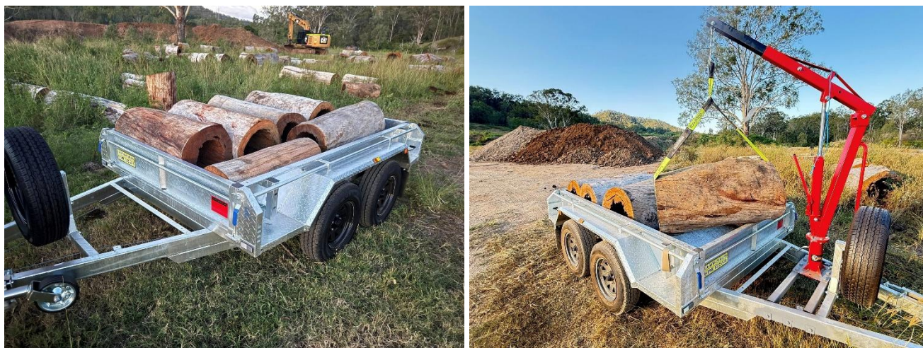
Loading 8 x 5 trailer at holding property for delivery to cluster sites. The use of a hand pumped dydraulic crane is advised.
